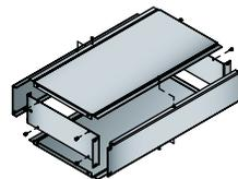
front and rear aluminum panels detach for simplified machining
