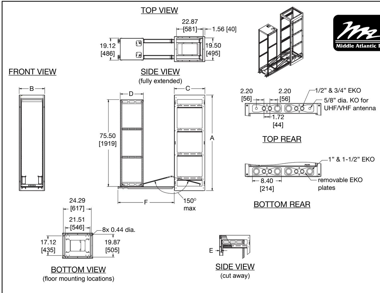
All dimensions in inches unless otherwise noted [Bracketed dimensions in millimeters]
