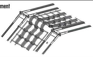
Service loop at center to allow full extension of CABLE CARRIER
