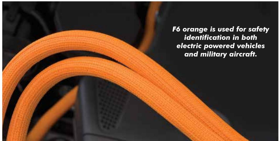
**F6 orange is used for safety identification in both electric powered vehicles and military aircraft.**
