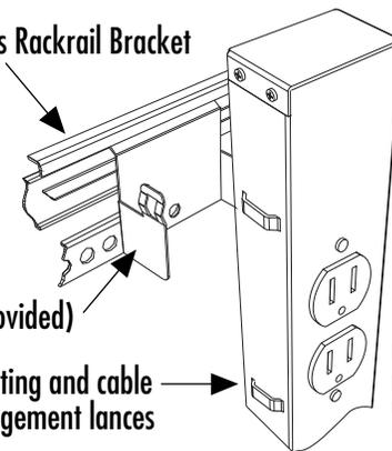
NOTE: Wood screws provided for attaching mounting clip to wood surfaces
