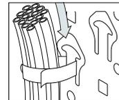
slide-on cable tie posts for dressing pre-assembled cable bundles
