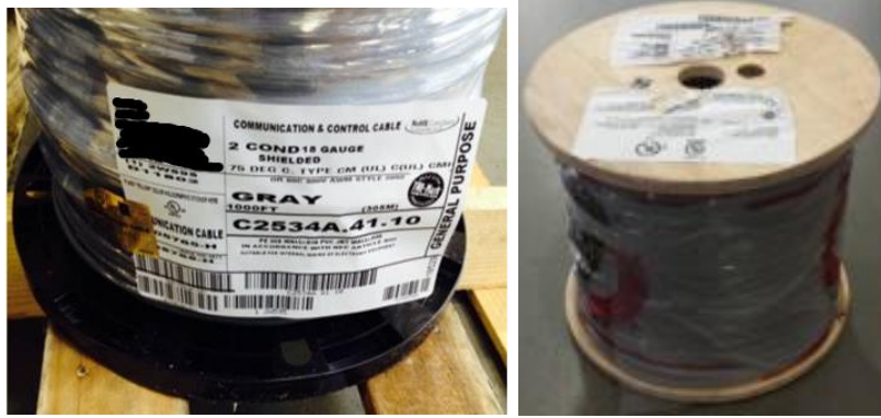
(Unacceptable labeling as the label might drop off) (Unacceptable Label as it was torn)
