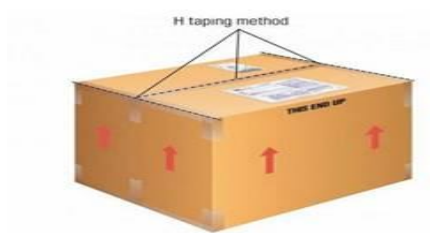
(Acceptable H Tape Sealing)
